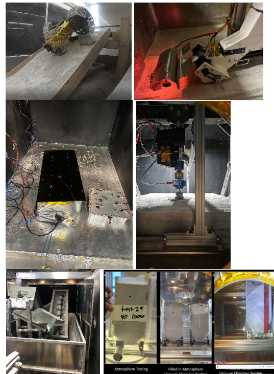
Figure 1: Various relevant environment tests for lunar technology development. Vehicle, construction, power, regolith transfer and wear testing shown in DTVAC as well as in regolith sandbox.
